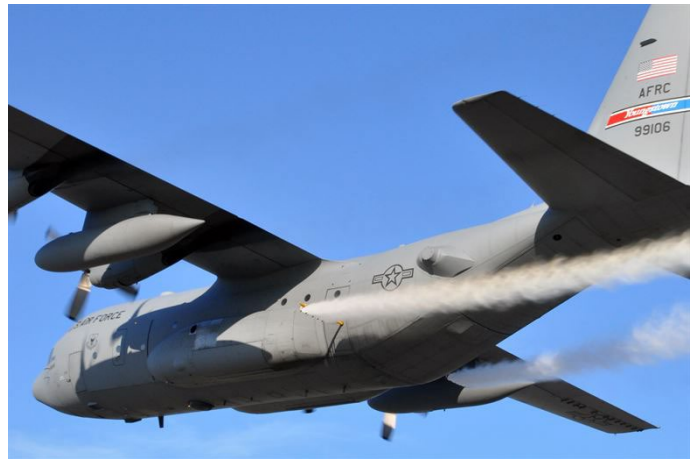
A Youngstown ARS modified C-130 Hercules aircraft simulates spraying pesticides during a field exercise
