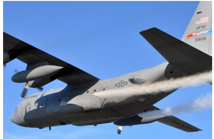
A Youngstown ARS modified C-130 Hercules aircraft simulates spraying pesticides during a field exercise
